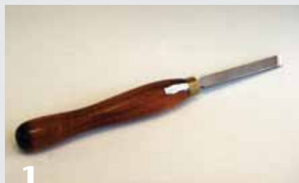
1 Madeleine's modified skew chisel has a mark on its handle to allow her to line up the tool in its proper position.
